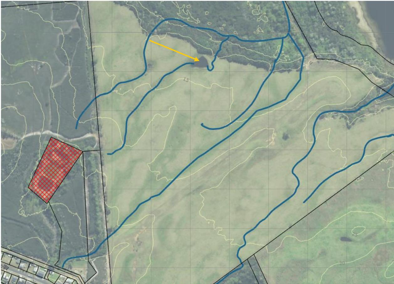
**Figure 1: The wastewater treatment plant (red cross hatching), 5m contours (light yellow) and approximate surface (and near surface) water flows in dark blue. The yellow arrow points to the small pond where water quality samples have been taken. Rotokawau Lake (west) is just visible in the top right hand corner.**
