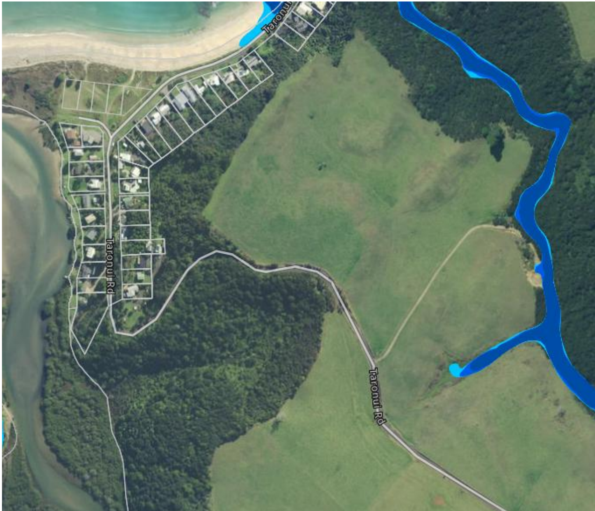
Figure 6. NRC Region Wide Flood Model, Flood Extent North at top of page, extract from NRC Maps
