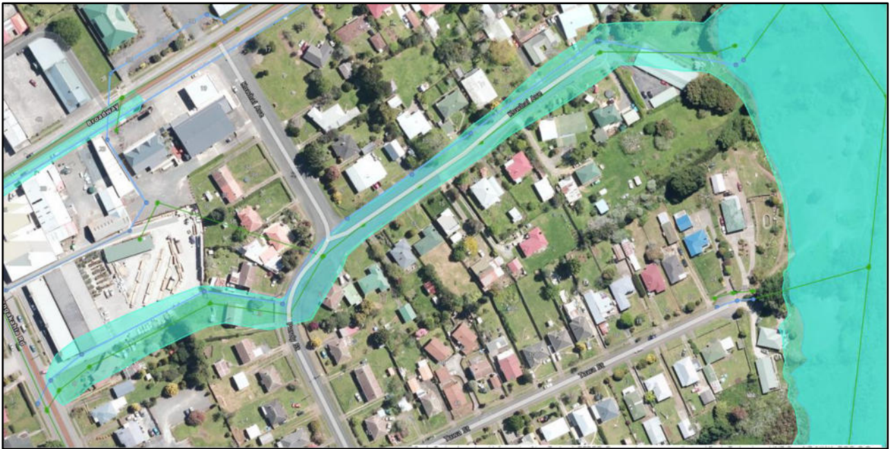
Figure 6 Downstream OLFP and Flooding extent
