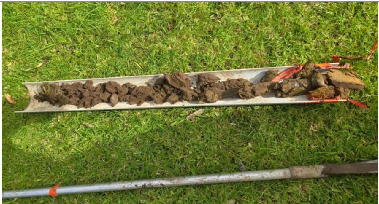
250mm sandy loam topsoil over sandy loam Class 4, (as per AC TP-58, Table 5.1)
