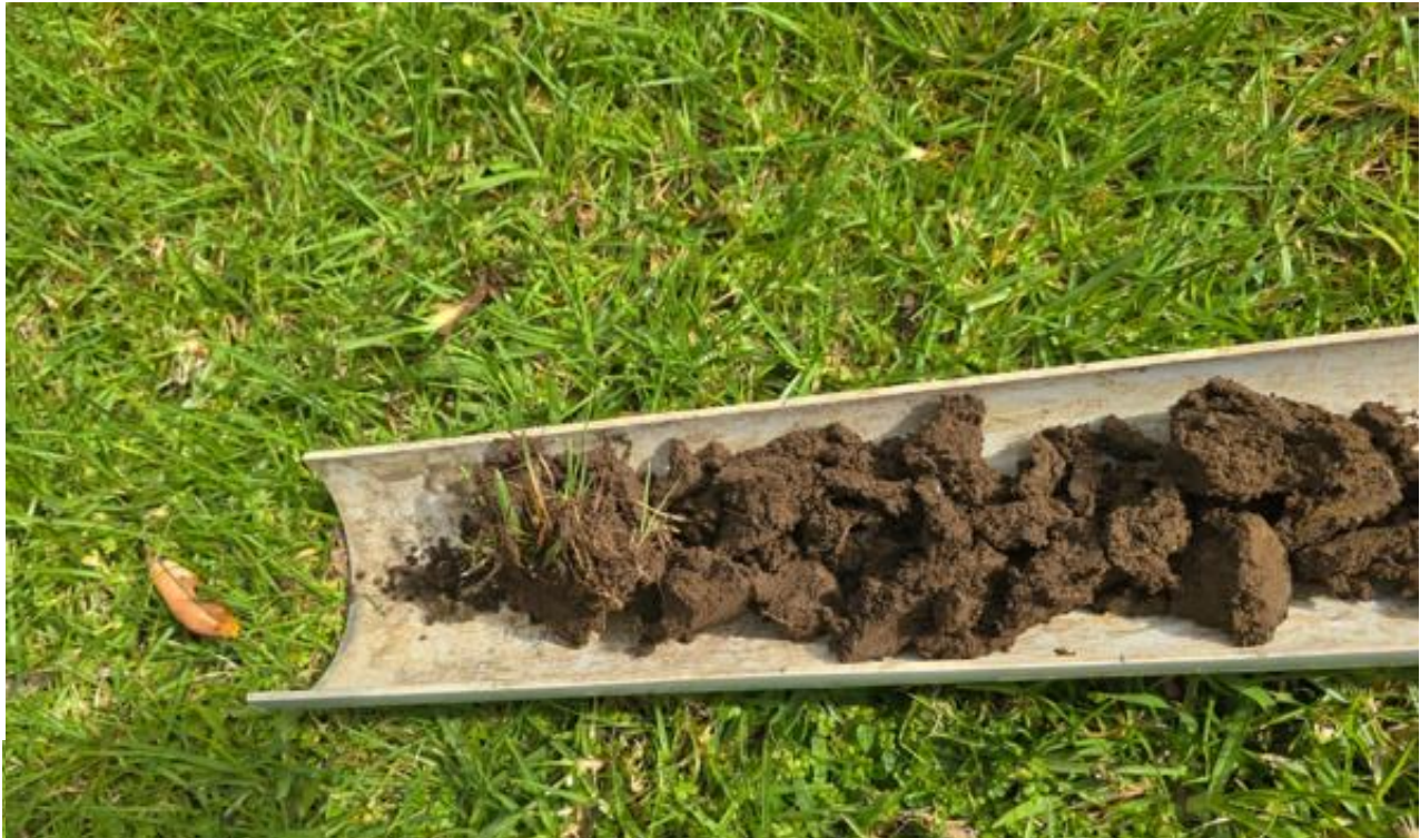
250mm sandy loam topsoil over sandy loam Class 4, (as per AC TP-58, Table 5.1)
