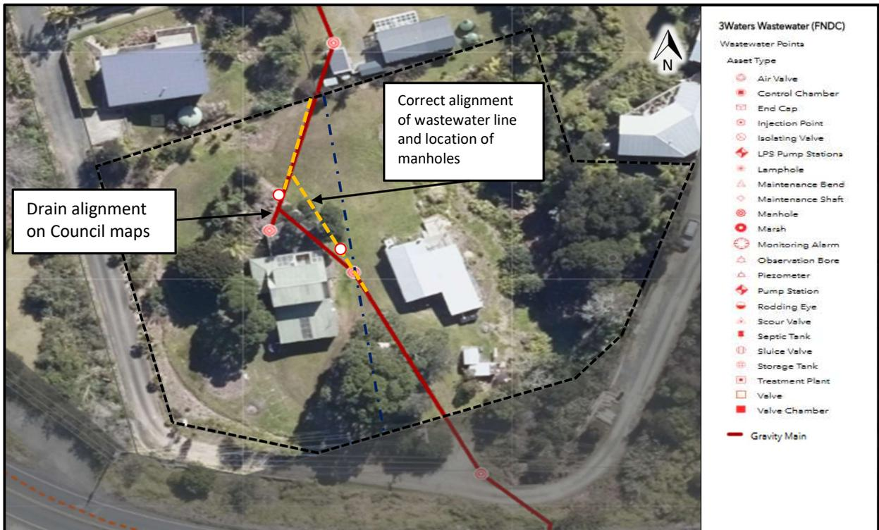
Figure 4: Existing wastewater network (Source: FNDC Water Services GIS service).
