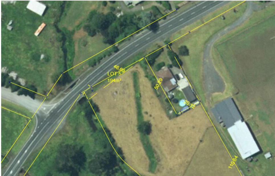
Figure 2: Survey map showing existing boundaries relative to the existing carriageway
