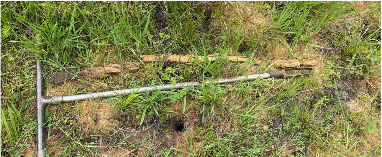
Photograph 2: Borehole showing 100mm of category 5, slightly moist, brown topsoil followed by category 6, slightly moist, orange, silty clay.
