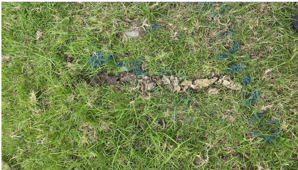
Photo 6: HA02 Core Samples (0-1.3m from left to right).
