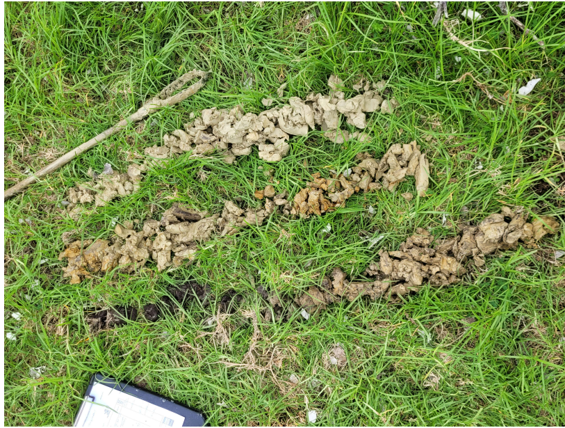
Photo 5: HA01 Core Samples (0-1m bottom row, 1-2m middle row, 2-3 top row).
