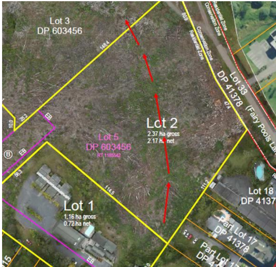
Figure 2: Overland Flow Path
