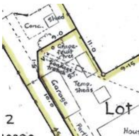
Figure 7 – Setback Breaches on Lot 1 [Source: Nigel Ross Surveyor]
