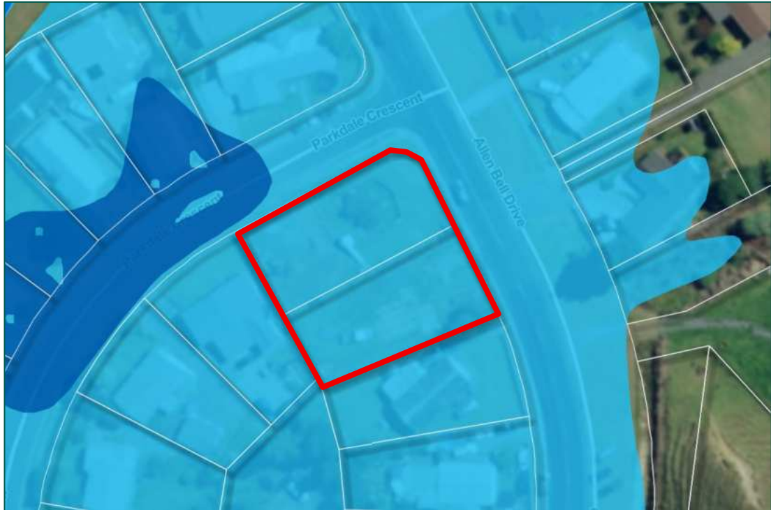
Figure 3. 100-year flooding as it applies to the subject site (outlined in red). Source: NRC Hazard Viewer.
