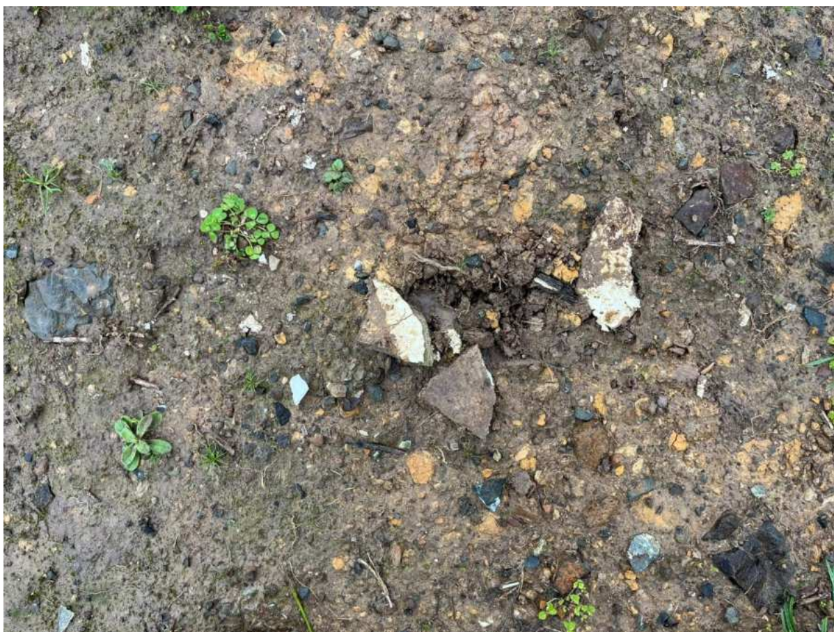
Photograph Appendix A.3: Potential ACM fragments on 61 Allen Bell Drive.
