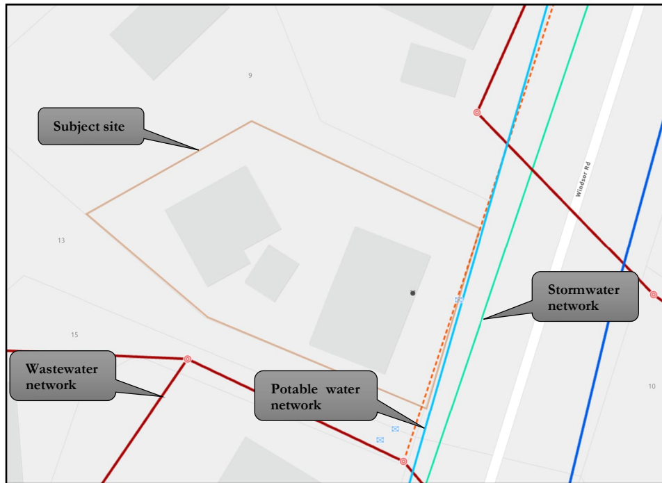
Figure 2: Three-waters infrastructure existing in the vicinity of 11 Windsor Road, Kaikohe (obtained from Far North District Council's GIS)
