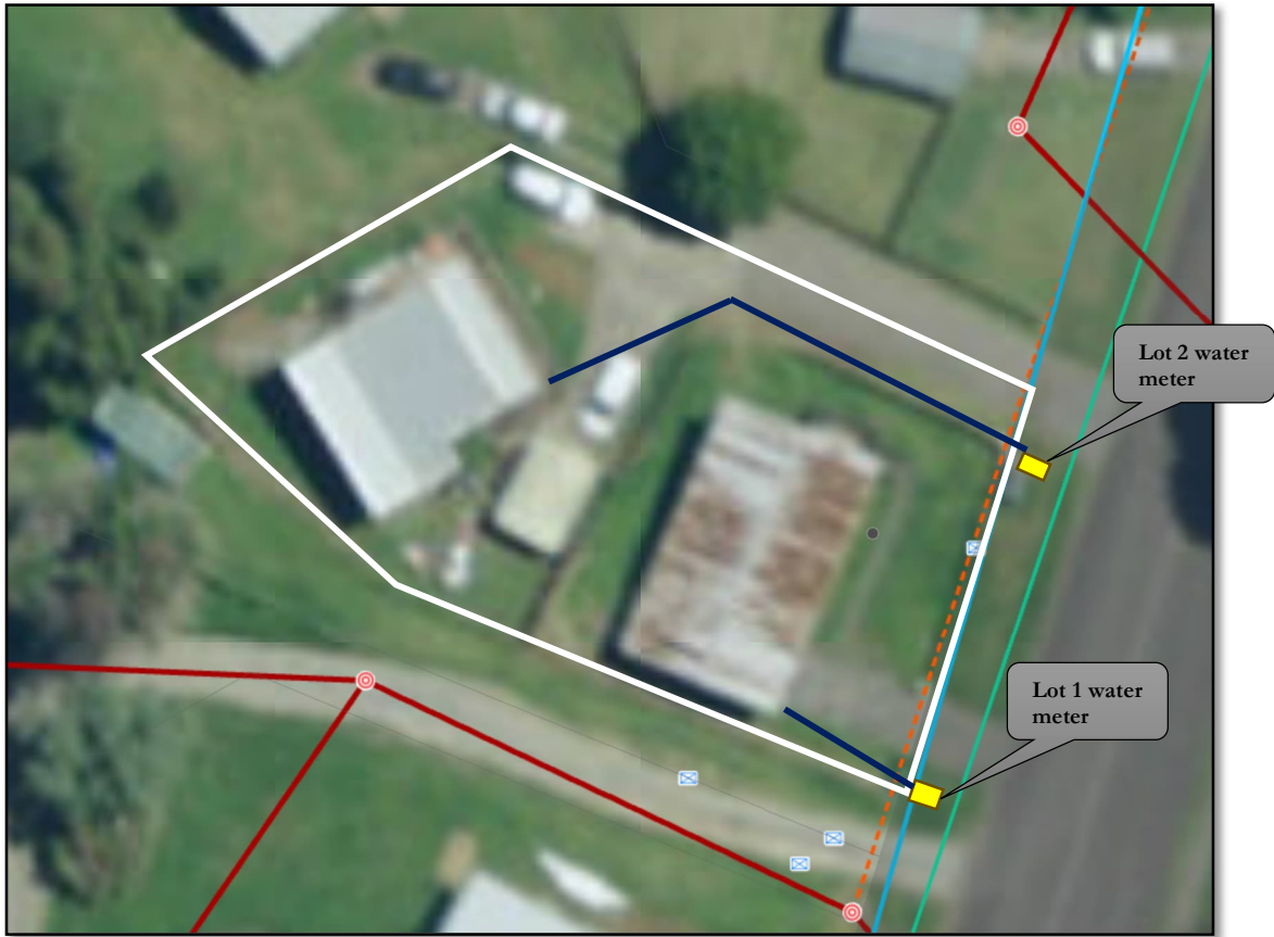
Figure 4: Location of water meters serving the site (possible layout of potable water pipe, no utility ground investigation conducted)
