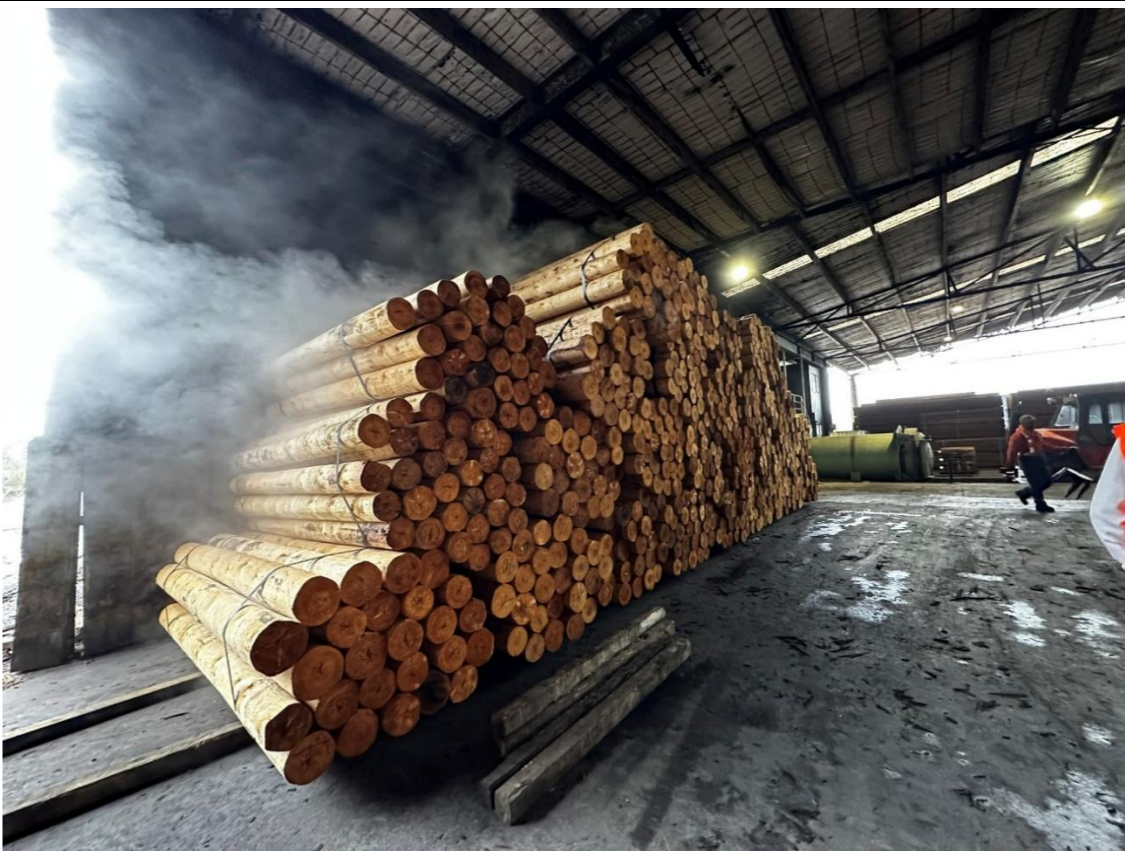
Photo 4: Freshly treated logs on the drip pad.
