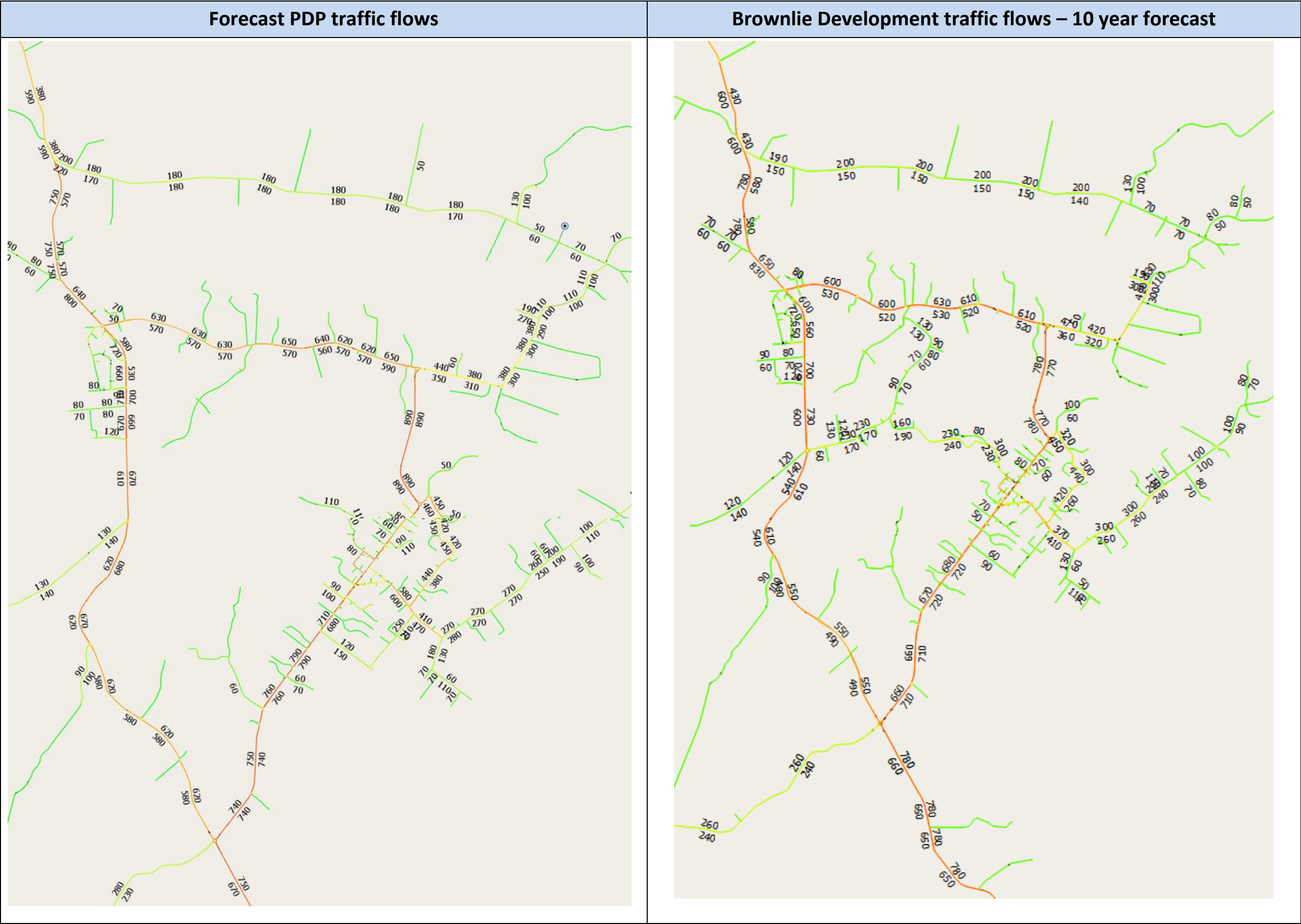
Figure 13: Comparison of forecast PDP and Brownlie Development (10 year scenario) traffic flows (vehicles) – Evening peak hour (4:30 pm to 5:30 pm)
