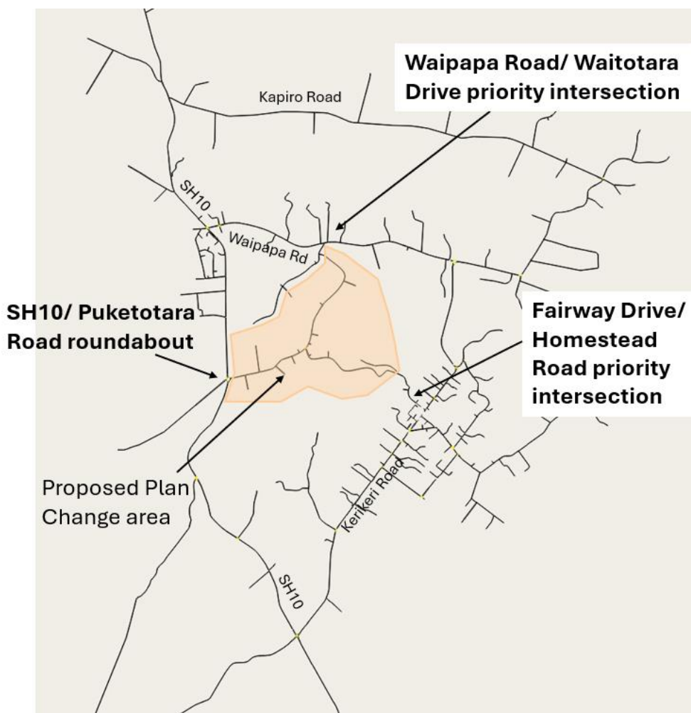
Figure 5: Kerikeri Transport Model extent and Proposed Plan Change area with proposed access points to the existing road network
