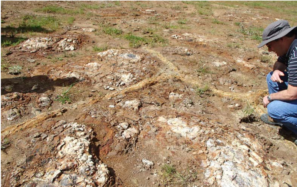
Photo 3: Infilled rock seams, irregularly oriented, at base of upstream quarry.
