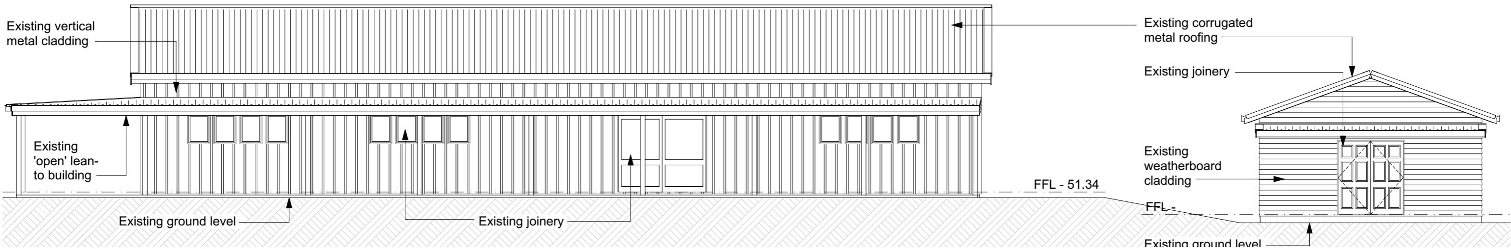
06 EAST ELEVATION - AS EXISTING
