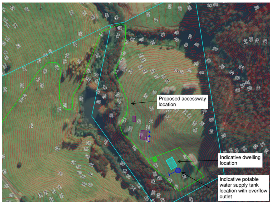
Figure 11: Indicative potable water supply tank with overflow outlet
