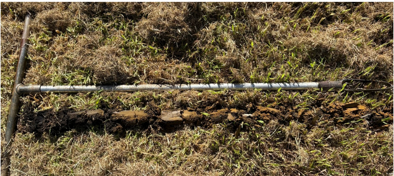
Photograph 2: Borehole showing 100mm of category 4, slightly moist, dark brown topsoil followed by category 5, slightly moist, orangey brown, silty clay to a depth of 1200mm.
