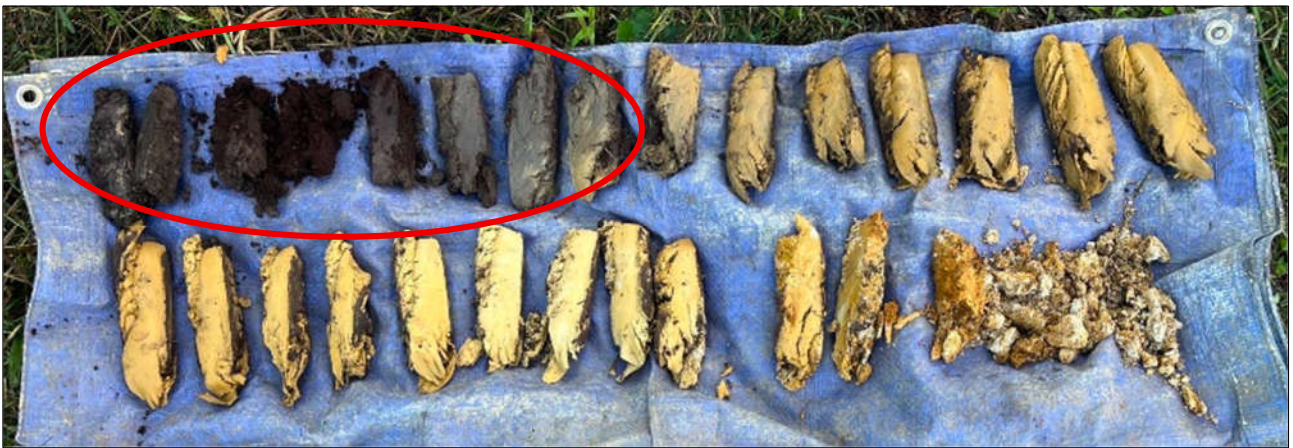
Figure 15: Site photograph of the HA02 soil arisings (0.0m to 2.1m). Red ring depicts the surficial fill and buried topsoil stratum.
