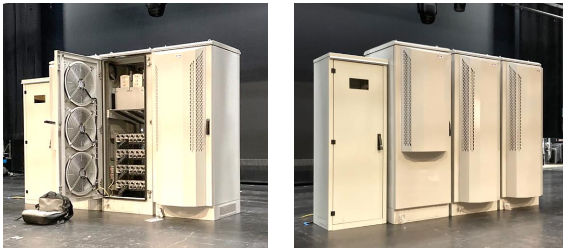
Figure 1 Cabinet group arrangement under test From left to right: Utility cabinet, PEB cabinet, Radio cabinet, Radio cabinet
