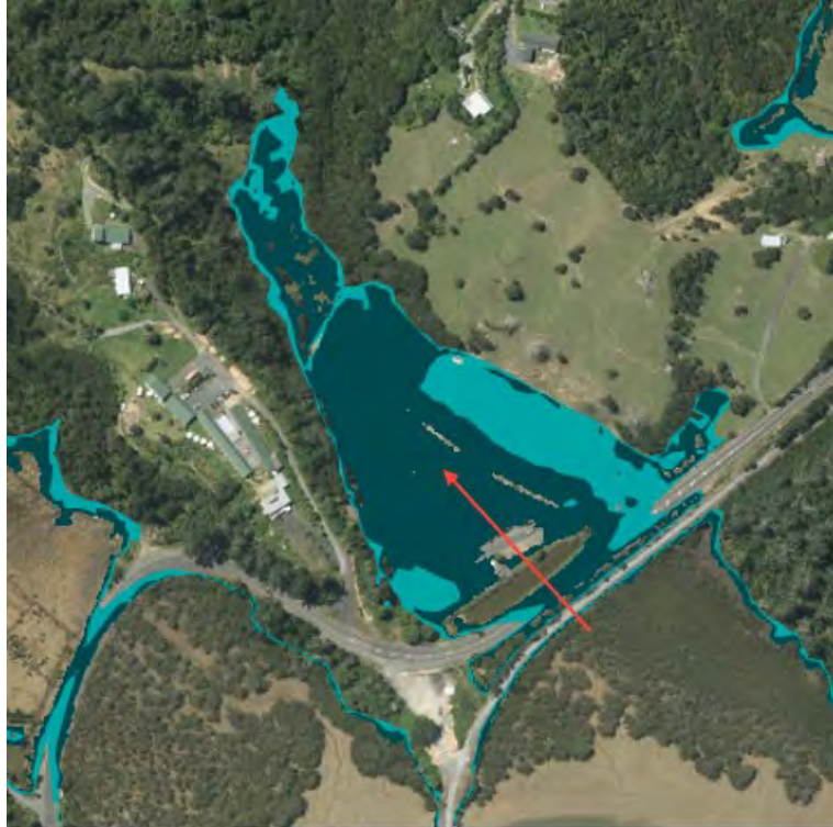
Figure 3-4 Current coastal flood model of the Commercial Estate (red arrow) under current flood (dark blue) and 1:50-year flood model (light blue).
