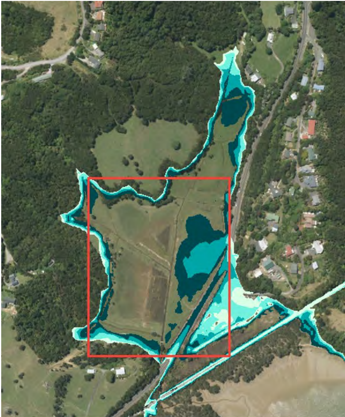
Figure 3-9 Current coastal flood model of the Marine Park (red square) under current flood models present extent (darkest blue), 1:50-year extent (second darkest blue), 1:100-year extent (second lightest blue), 1:100-year + RSL (lightest blue).
