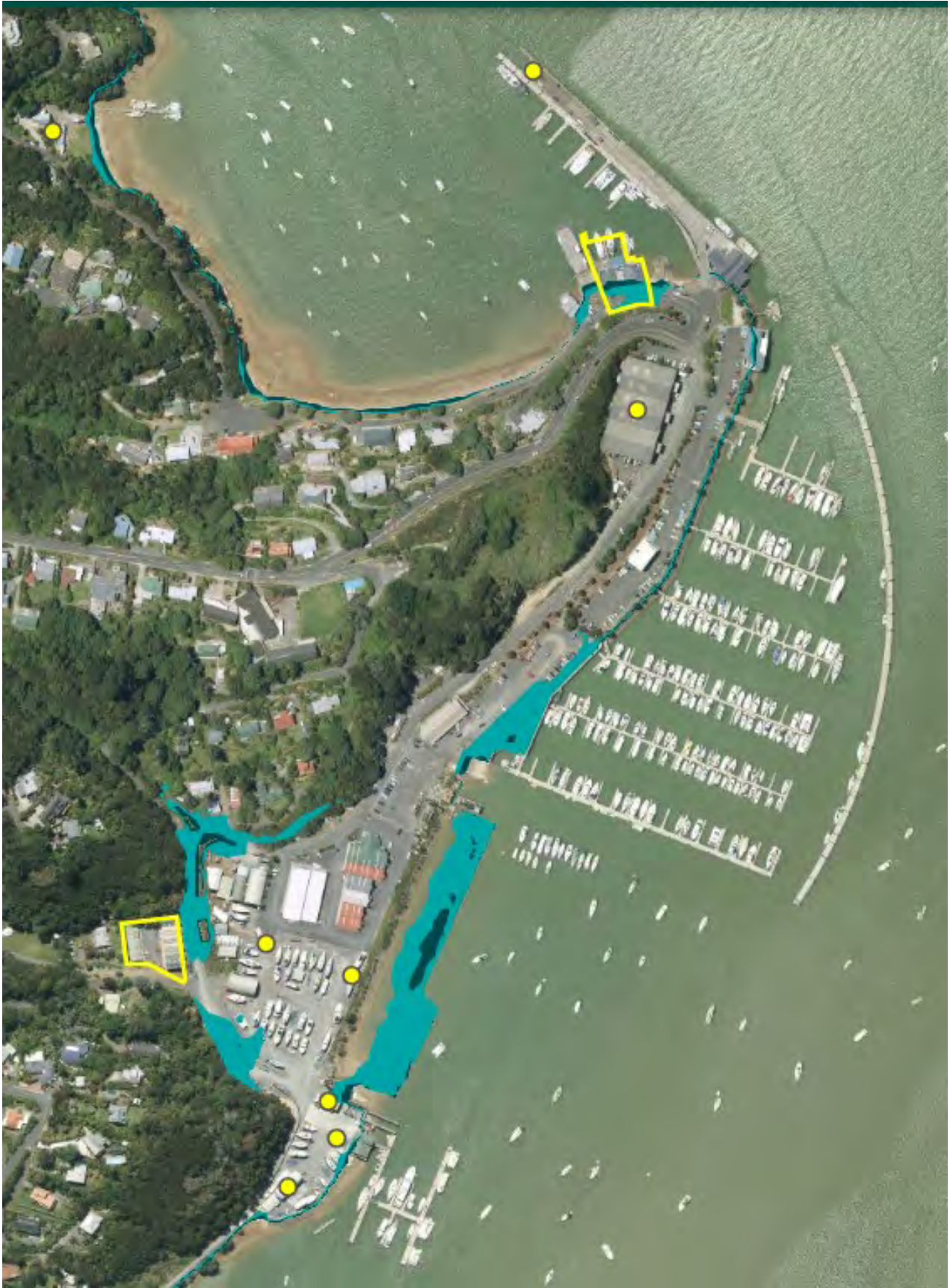
Figure 3-2 Flooding Hazard Zones of Bay of Islands Marina (dark blue = current coastal flooding zone, light blue = 50-year coastal hazard flood zone, HAIL Sites have been highlighted in yellow, Source: NRC).
