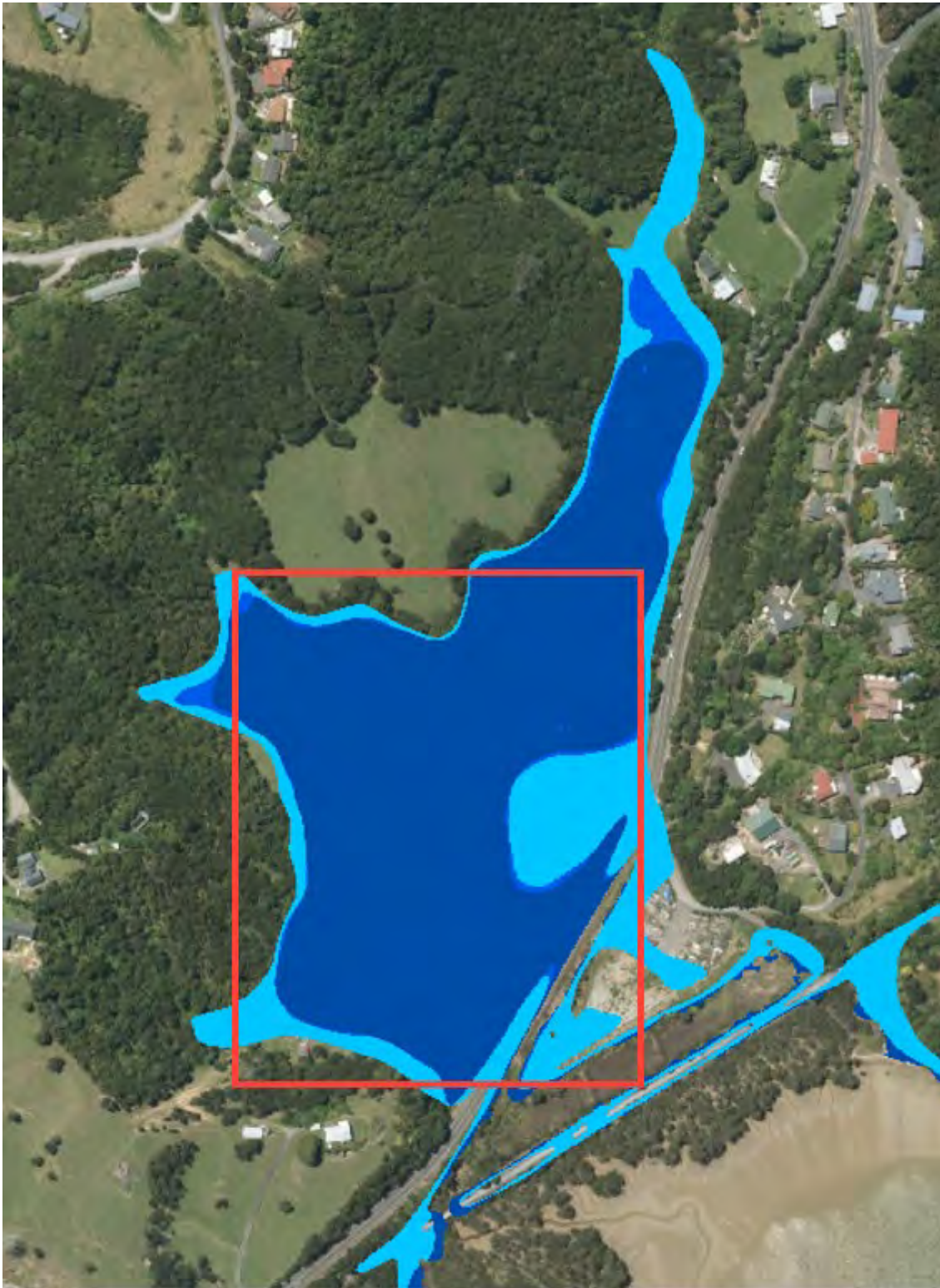
Figure 3-8 Current River flood model of the Marine Park (red square) under current 1:10-year extent (darkest blue), 1:50-year extent (middle blue), 1:100-year CC extent (lightest blue).
