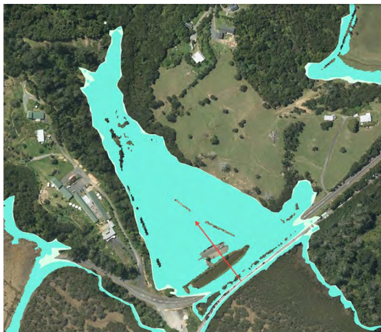
Figure 3-5 Coastal flood model of the Commercial Estate (red arrow) under a 1:100-year (darker blue) and 1:100-year + RSL scenario (lighter blue).
