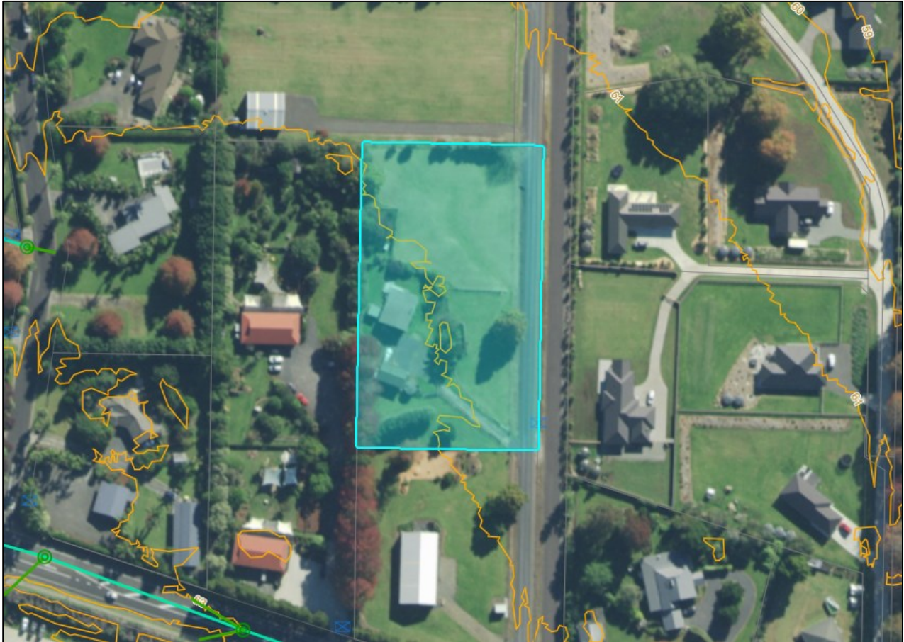
Figure 2: Snip from FNDC Water Services Map showing site boundary (cyan), 1m contours (orange), public potable water (blue) and public stormwater (green)
