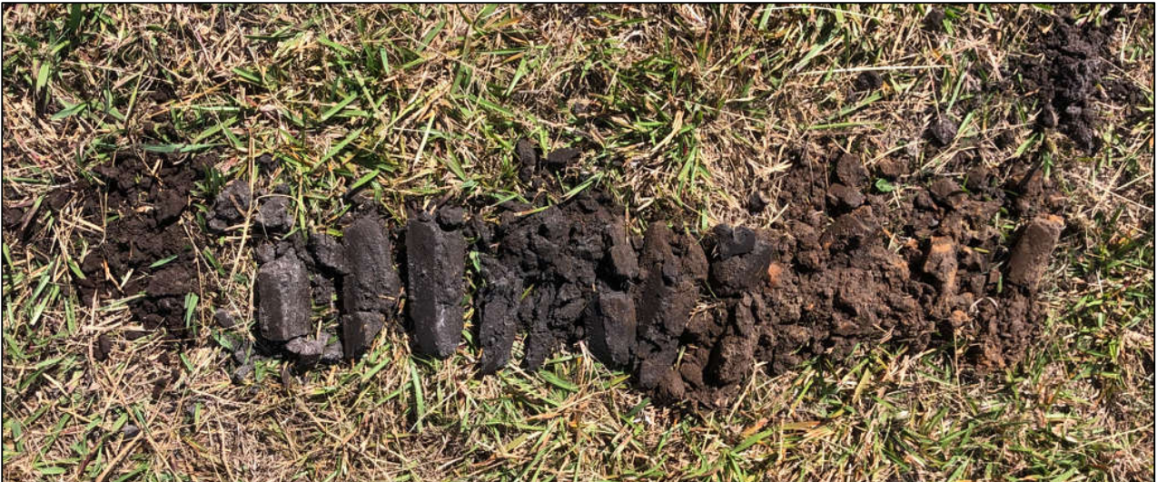
Figure 7: Site photograph of HA01 which were typical of the soil arisings encountered (0.0m to 0.95m).
