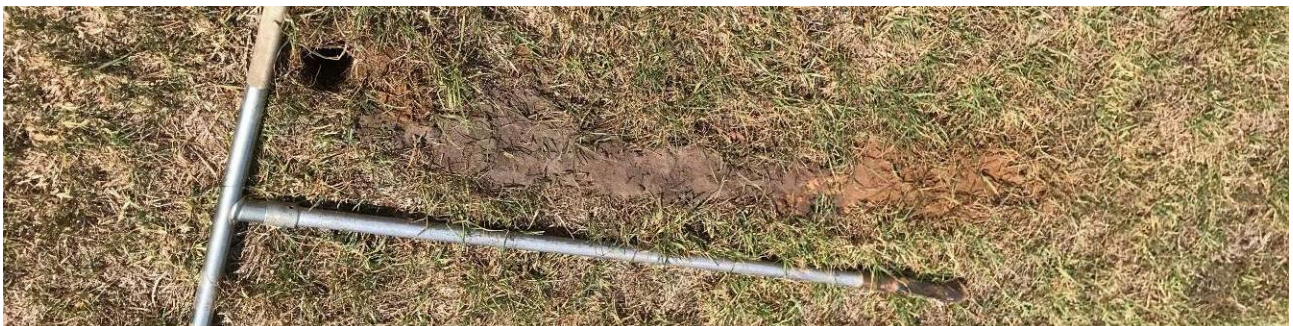
Photograph 5: Showing 300mm of category 3, dry, light brown, silty SAND followed by category 3, slightly moist, reddish brown, silty SAND.
