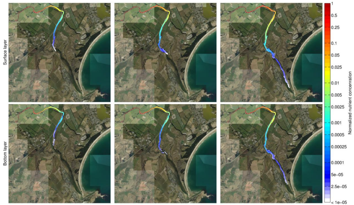
Figure 2: Waikouaiti Estuary modelling. Relative concentration of river nutrients after 24H of continuous release from Orbell's Crossing under the three flow states considered during spring tide
