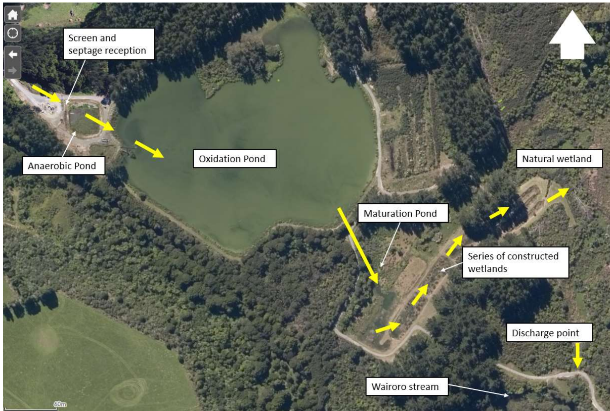
Figure 2-1 Kaikohe WWTP detailed process of effluent treatment onsite, Cumber Road, Kaikohe. Image taken from WDC GIS Maps 2021.
