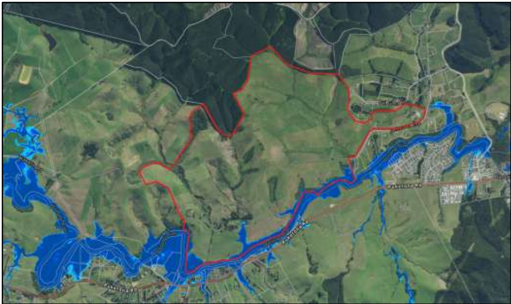
Figure 6: River Flooding Hazard Overlay (Source: NRC Maps).
