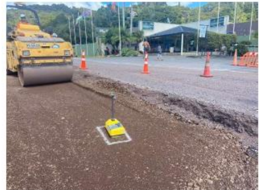
Kings Rd – Testing on subbase later – Nuclear Densometer
