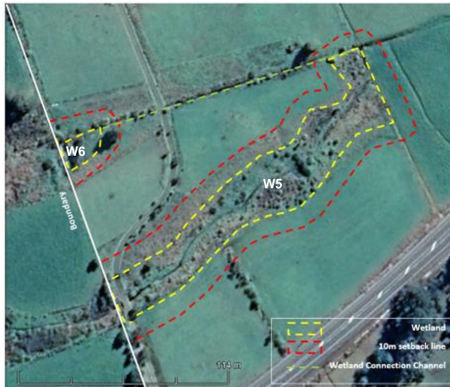
Figure 7: Wetland area outlined in yellow, with minimum 10m buffer planting in red. An existing drain connects the two wetland areas (green). The large wetland (W5) is connected to more extensive wetlands to the west as is the smaller one demarcated (W6).
