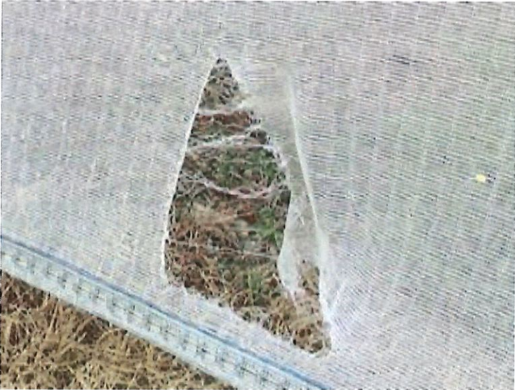
Artificial structures normally use plastic cloth, such as HDPE polyethylene – the plastic cloth degrades over time, releasing microplastic into the environment
