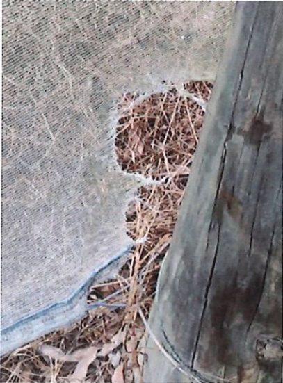
Artificial structures normally use plastic cloth, such as HDPE polyethylene – the plastic cloth degrades over time, releasing microplastic into the environment
