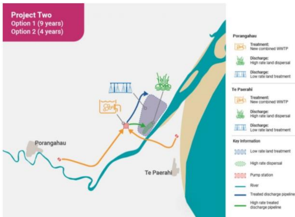
Figure 11 – Proposed Future Wastewater Network 10
