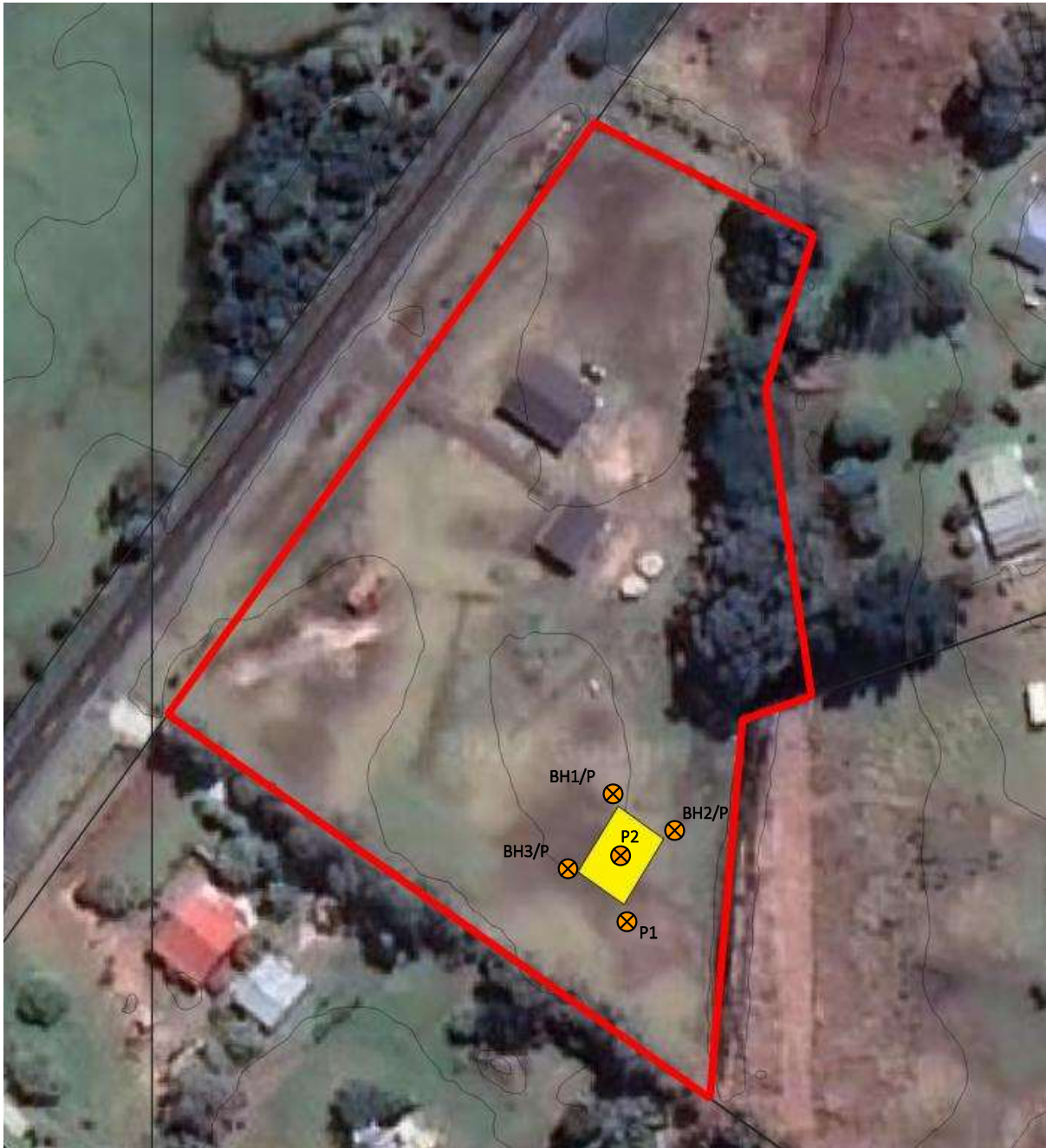
Figure 2. Geotechnical Test Location Plan
