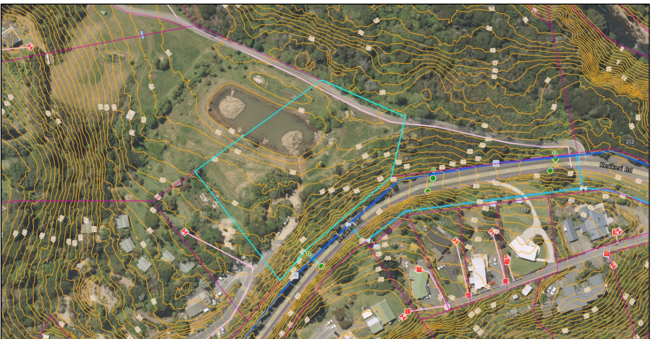
Figure 1: Aerial Snip from FNDC Maps Showing Site Boundaries (cyan), Public Stormwater (green), Public Wastewater (red), Public Potable Water (blue) & 1m Contours (yellow)
