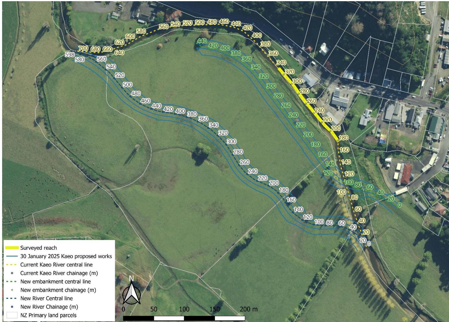
**Figure 5-1: Proposed works to divert the Kāeo River and construct a floodwall (embankment).**
