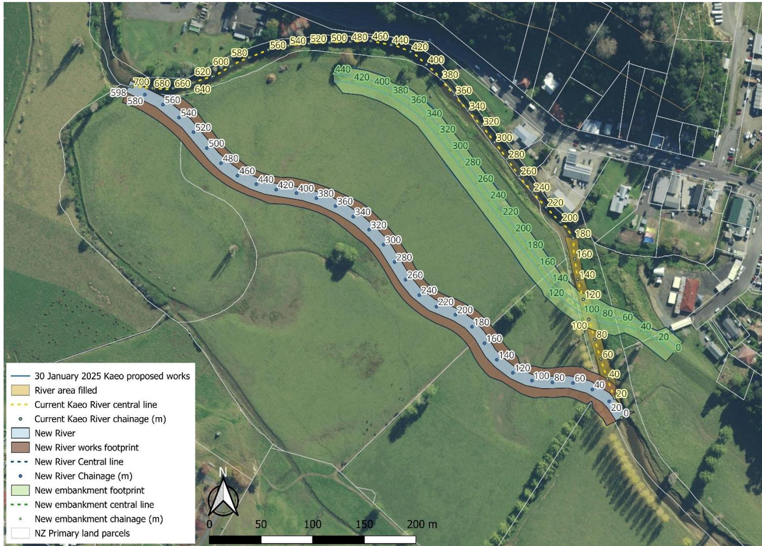
**Figure 5-2: Areas of proposed works to divert the Kāeo River and construct a floodwall (embankment).**
